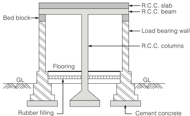
**Fig. Composite Structure**
